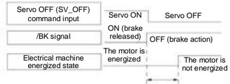
**Important** When an alarm occurs, regardless of this setting, the servo motor immediately enters a non-energized state. At this time, the machine sometimes moves before the brake is activated due to the dead weight or external force of the movable part of the machine.
