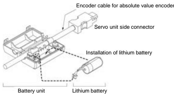
4. Cover the outer cover of the battery unit.
