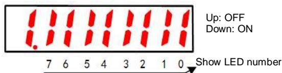
The input signal OFF corresponding to the LED number is displayed: the upper segment lights up
