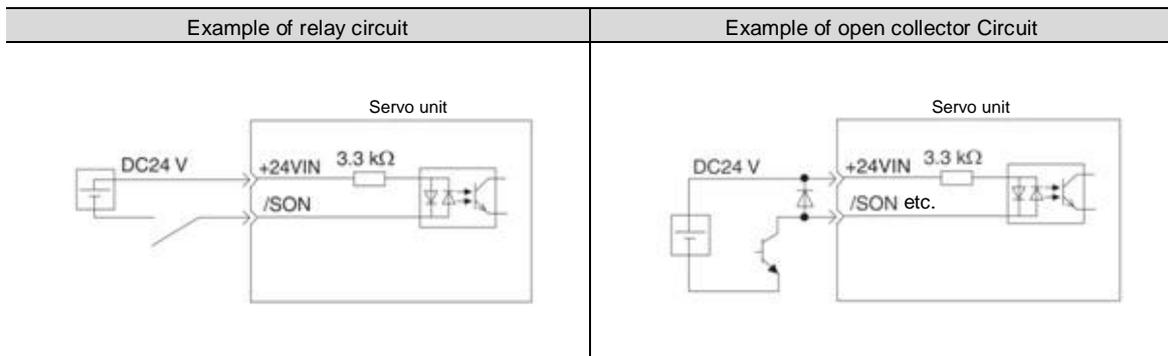
(Note) The external power supply (DC24 V) must have a capacity above 50 mA.
