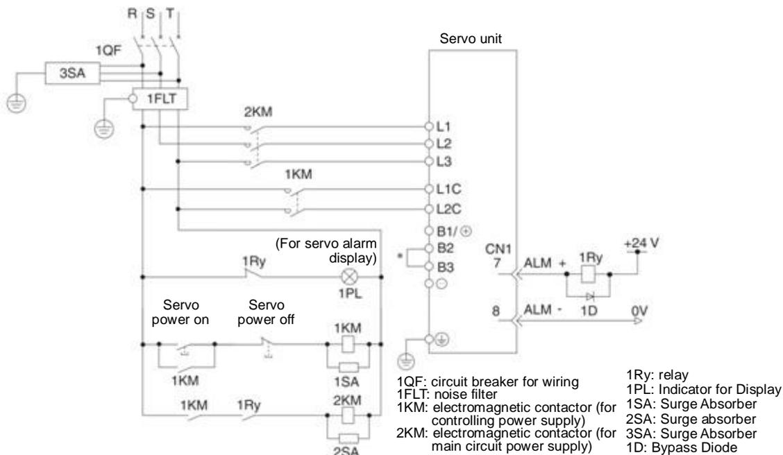
\* HSD7-28D□□, HSD7-40D□□ No built-in resistor, no short circuit between B2 and B3. Please do not short-circuit.
