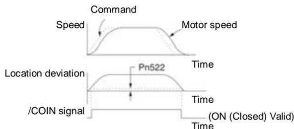
(Note) If the set value is too large and the deviation during low-speed operation is small, a constant /COIN signal may be output. When outputting the signal, please lower the set value until the signal is no longer output.
