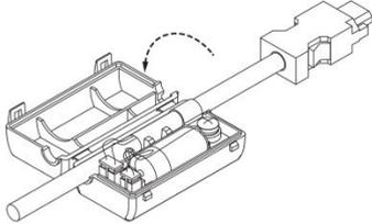
3. Remove the used battery and install the new battery.
