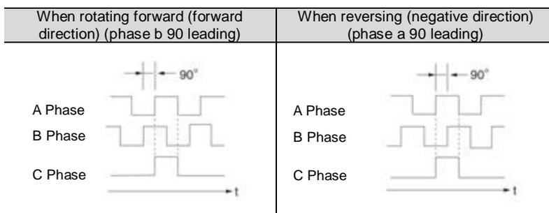
(Note) The pulse amplitude of the origin within the encoder 1 coil varies depending on the number of encoder divided pulses (Pn212) and the encoder output resolution (Pn281). Same amplitude as phase A.
