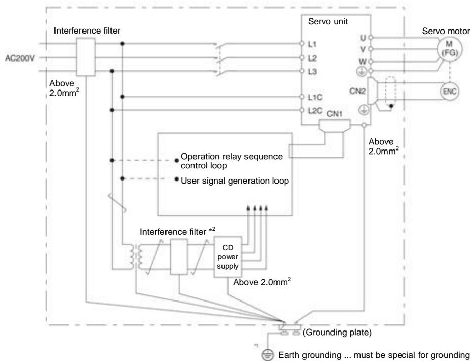
\*1. Please try to use a thick wire of more than 2.0 mm<sup>2</sup> for grounding (flat braided copper wire is more suitable).
