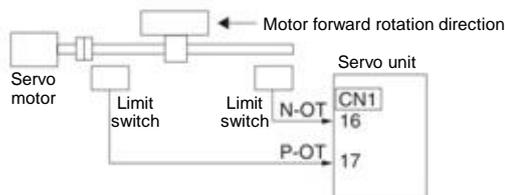
Rotary applications such as round tables and conveyors do not require over-travel prevention function, and there is no need to wire the over-travel prevention input signal at this time. The following is a description of the parameter setting related to the over-travel prevention function.
