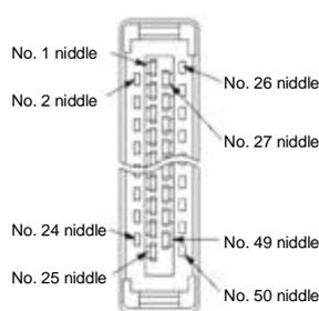
The appearance when the connector housing is not installed as seen from the arrow direction is as follows.
