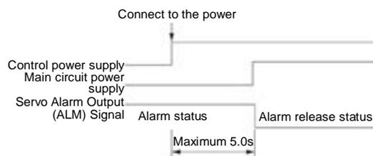
sequence control. Switch on the main circuit power supply after ALM signal OFF (alarm cleared).
