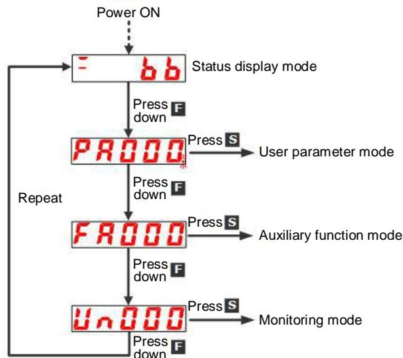
**补充说明** After setting Pn52F (monitoring display when power is turned on), the display content after power is turned on can be set in monitoring display (non-state display). Please set the un number to be displayed when the power is turned on in Pn52F.
