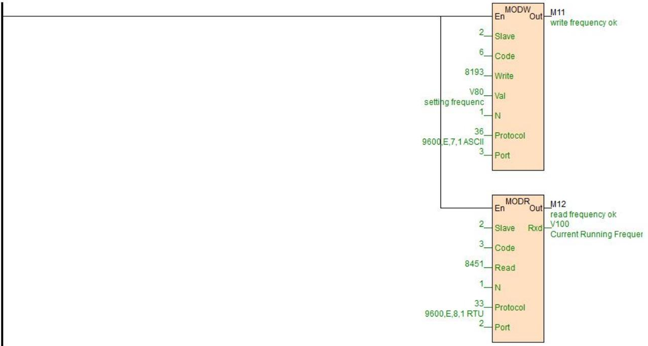
Port = 3, in this example, it indicates the communication port of AE-1C. 8193 can be quickly entered, such as put the mouse on the "Write" terminal, then it can directly enter 0x2001.
