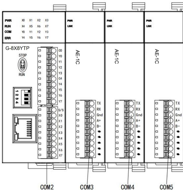
When the communication module is expanded, the communication port closest to the MPU is COM3, next is COM4 and last is COM5. The position of communication module can be random, and the communication port number can be viewed in the hardware configuration, as shown in the figure below:
