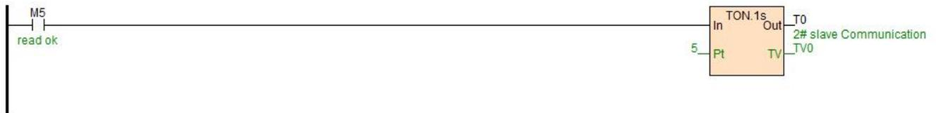
Communication disconnection time can be set according to the actual, the above when M5 is more than 5 seconds in OFF state, T0 coil will indicate communication disconnection alarm.
